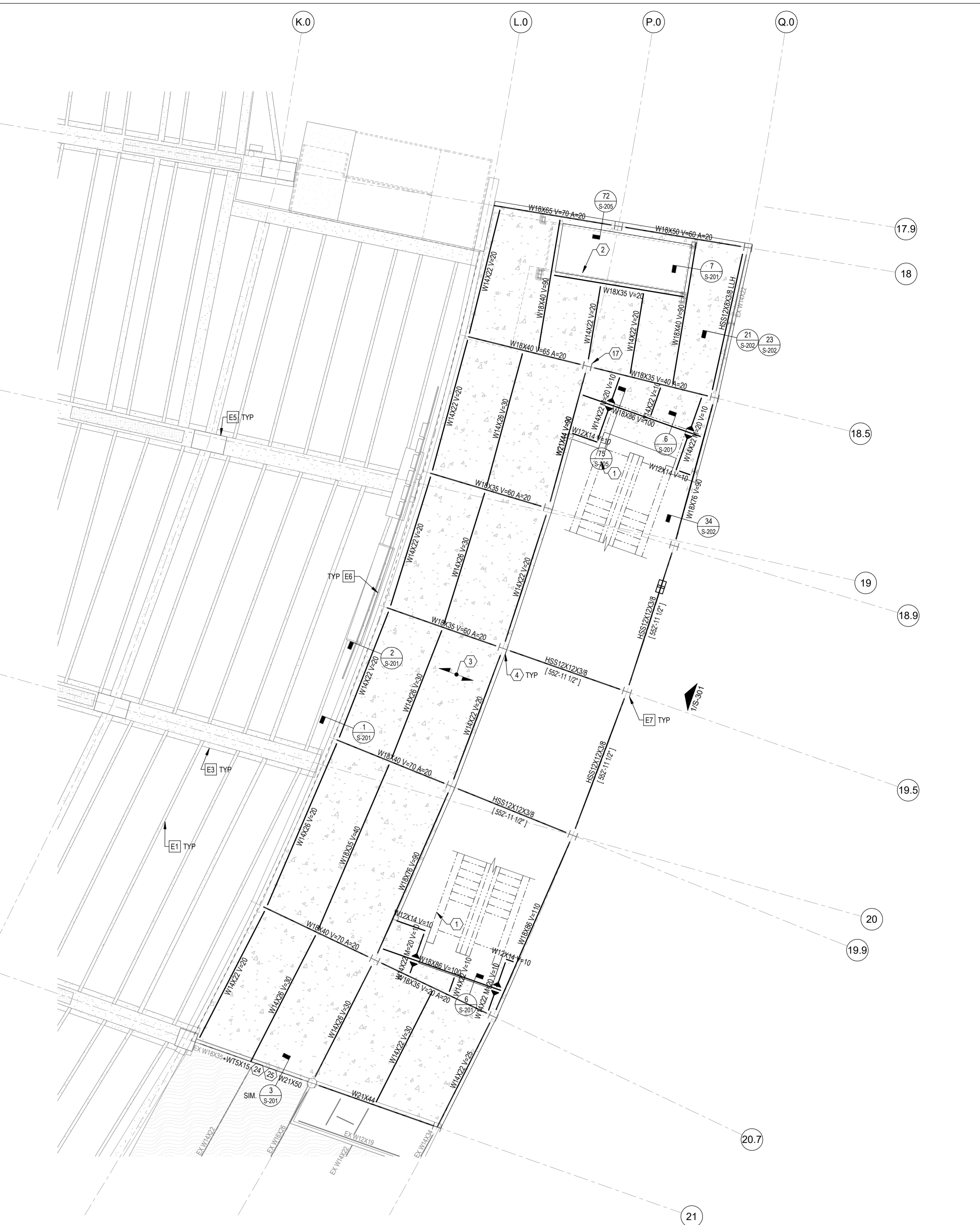
SECTOR 4 - T/SLAB = 553'-6"± U.N.O. 3 LEVEL 500 FRAMING PLAN S-103 1/8" = 1'-0"
