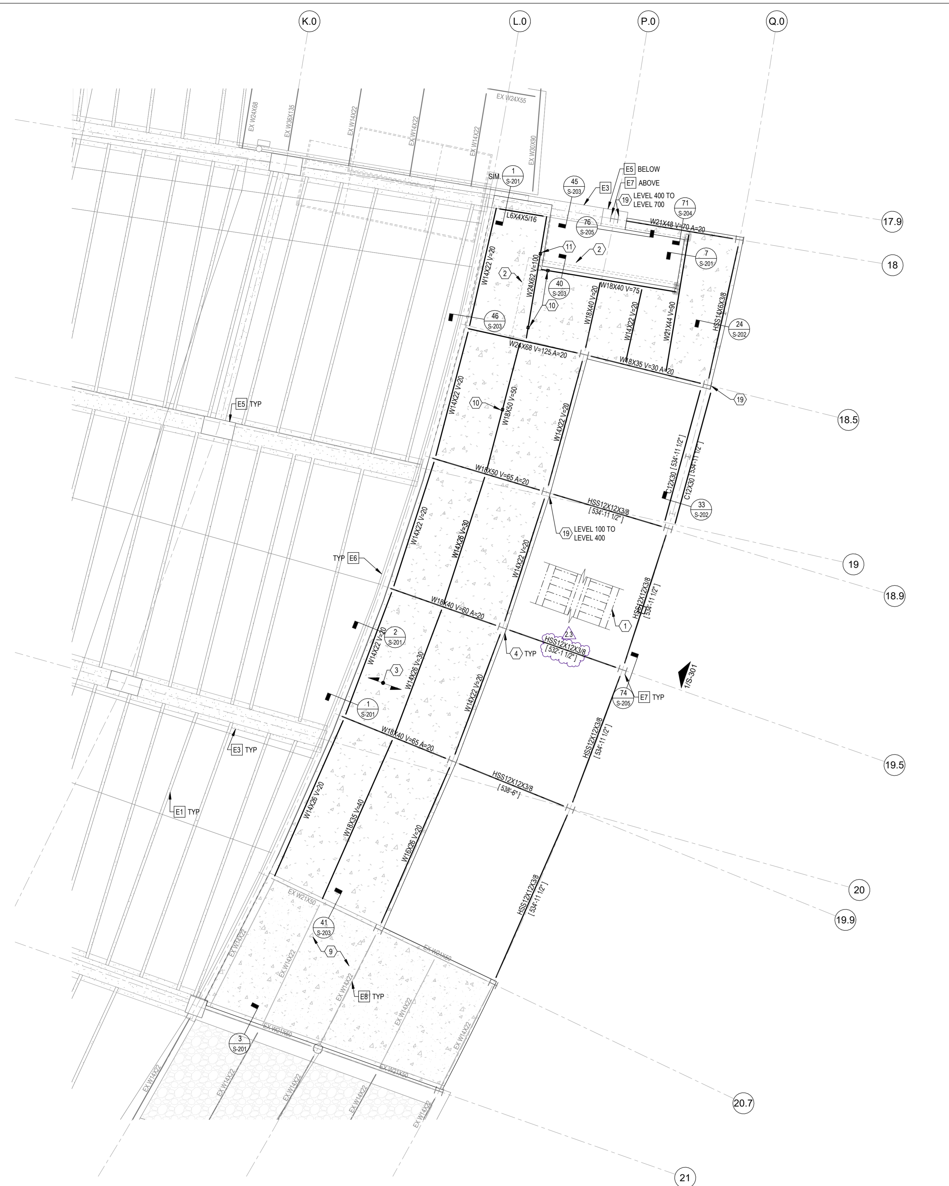
SECTOR 4 - T/SLAB = 535'-6"± U.N.O. 1 LEVEL 400 FRAMING PLAN S-103 1/8" = 1'-0"
