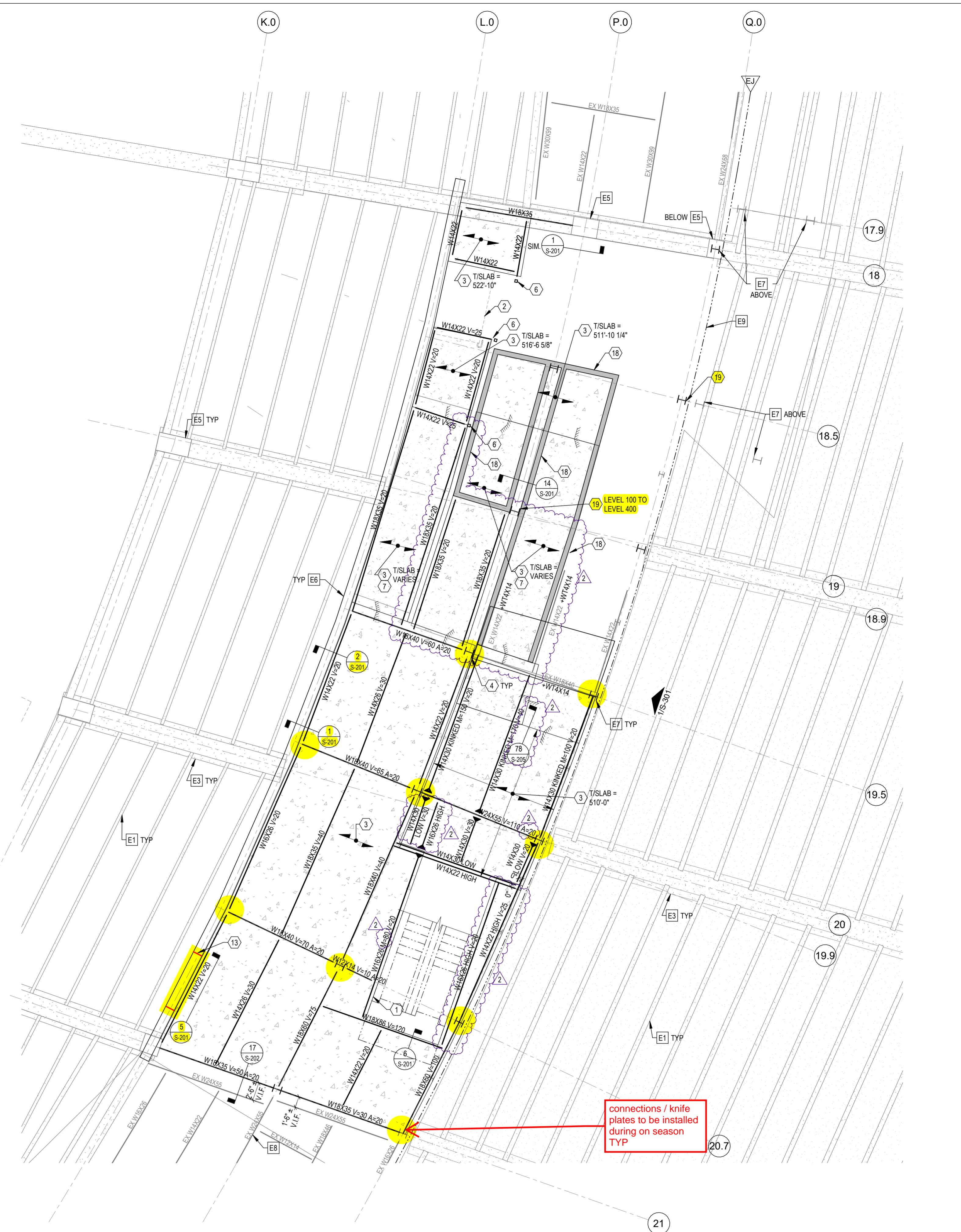
SECTOR 4 - T/SLAB = 515'-0"± U.N.O. 2 LEVEL 300 FRAMING PLAN S-102 1/8" = 1'-0"
