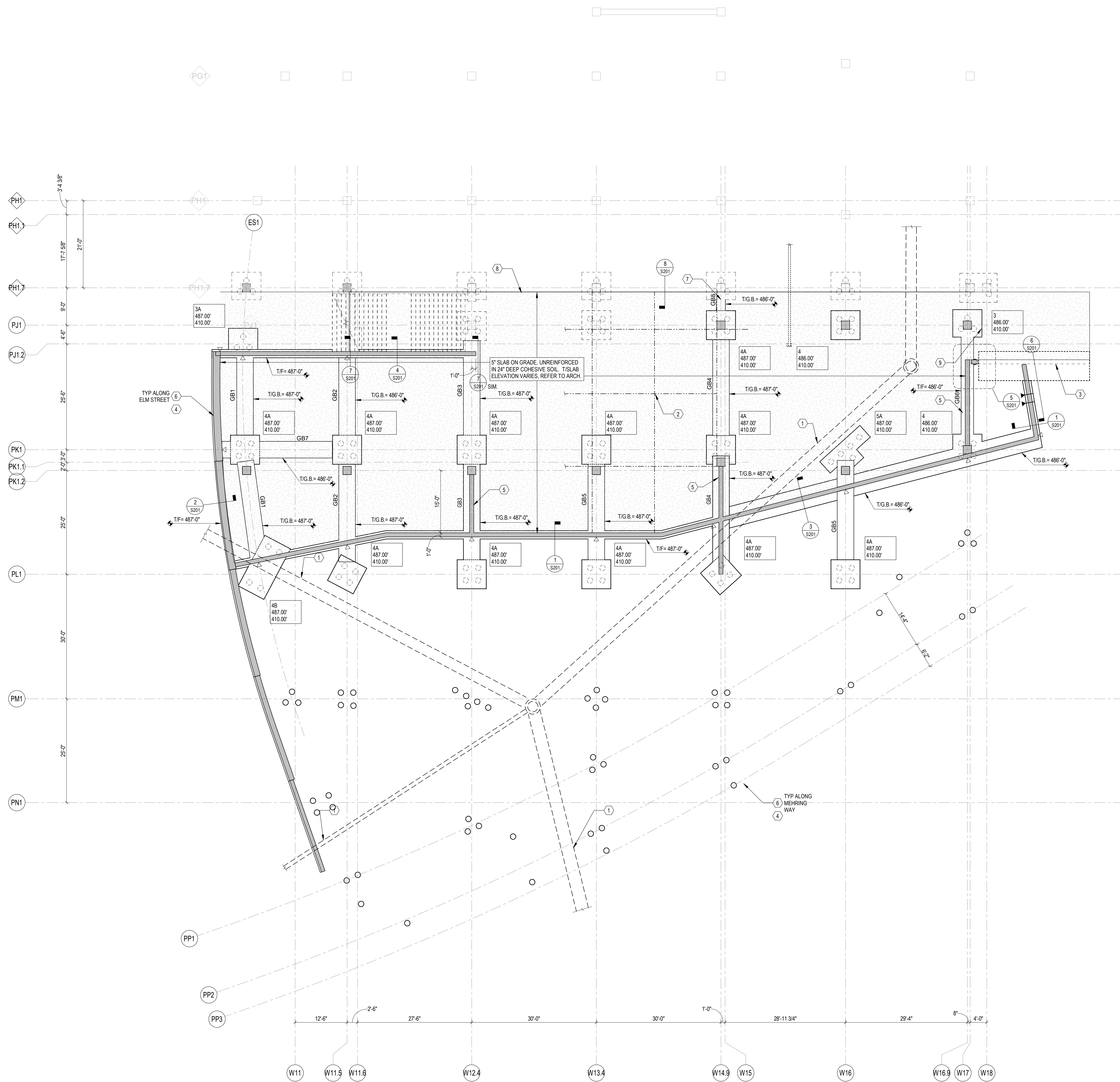
1 LEVEL 1 FOUNDATION PLAN S101 3/32" = 1'-0" NORTH
